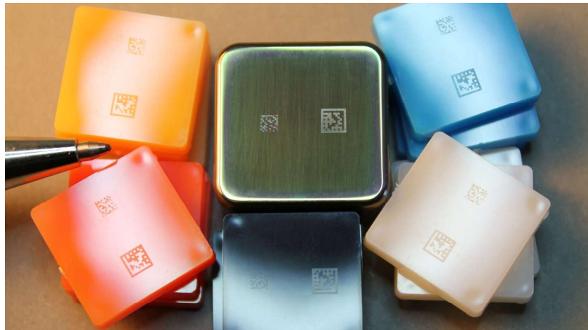
Tool insert, showing 2 microstructure barcode areas, surrounded by molded parts. 10x10 GS-1 Datamatrix. Side length is 2.5 - 3.0 mm. Smaller and larger is feasible. Any information content. Machine-readable.
